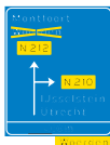
K9 Diversion with alternative route shown on an advance warning panel for a non-motorway highway
